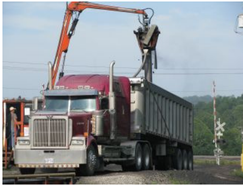
Coal sampling at wharf
